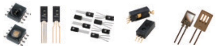
HIH6130/6131 Series HIH-4000 Series HIH-4020/4021 Series HIH-4030/4031 Series, HIH-5030/5031 Series HCH-1000 Series
