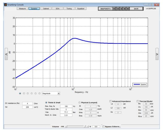
Figure 8. Smart Amplifier GUI Pop-Up
