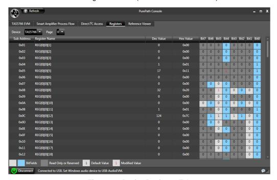
Figure 11. Device Registers Tab
