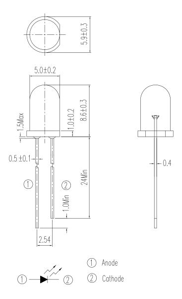
Note: Tolerances unless dimensions ±0.25mm
