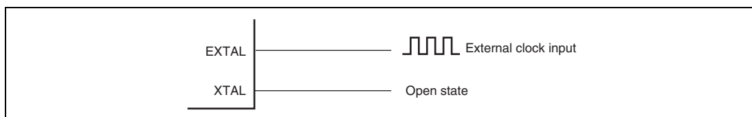
Figure 4.4 Example of External Clock Connection
