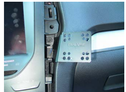
Mount installed showing screw location
