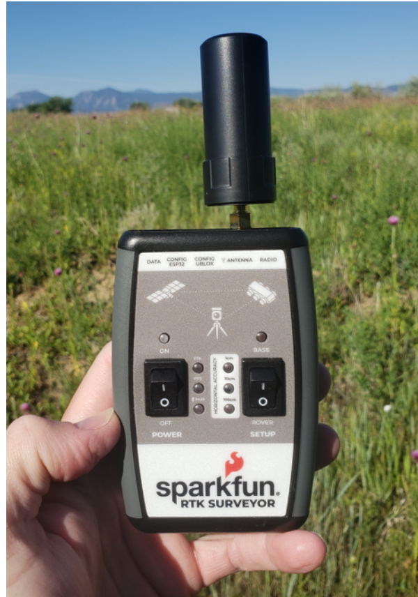
Dangerous Antenna Configuration
