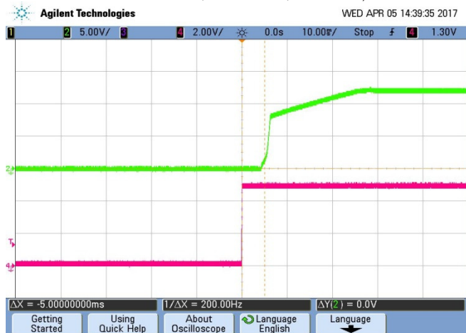
On/Off Enable Delay (Vin = 12V Vout= nom Iload =0A Cload = 200μF CH2: Vout; CH4: Enable; Ta=+25°C)
