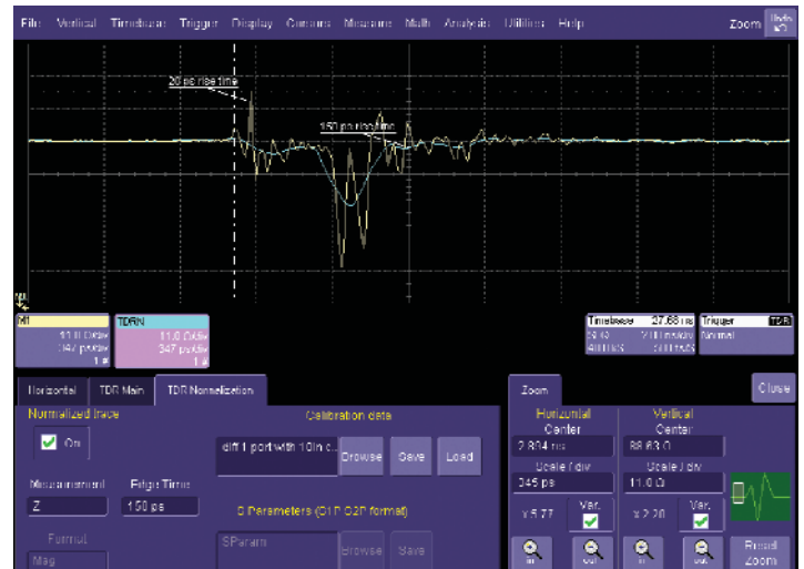
Calibrated impedance measurements are available with selectable rise time. This feature provides compliant impedance measurements of connectors, cables, and backplanes.
