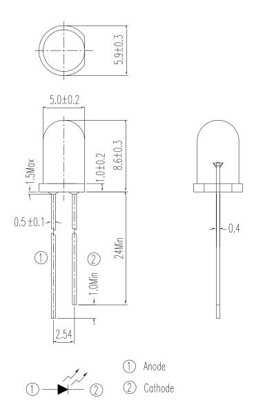
Note: Tolerances unless dimensions ±0.25mm
