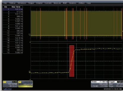
Use WaveScan to search for and identify anomalies on analog or digital signals.
