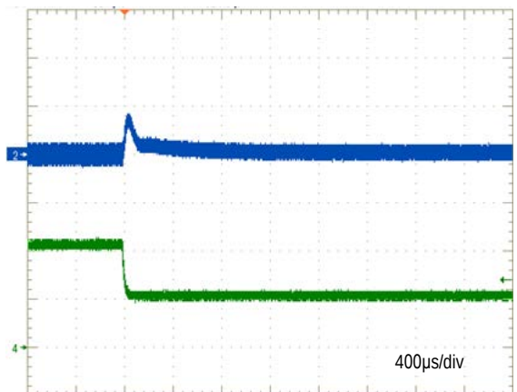
Transient Response (V in =48V, I out =2.125A to 1.06A, Ta=+25°C) Ch2=V out , 200mV/div, Ch4=I out , 1A/div
