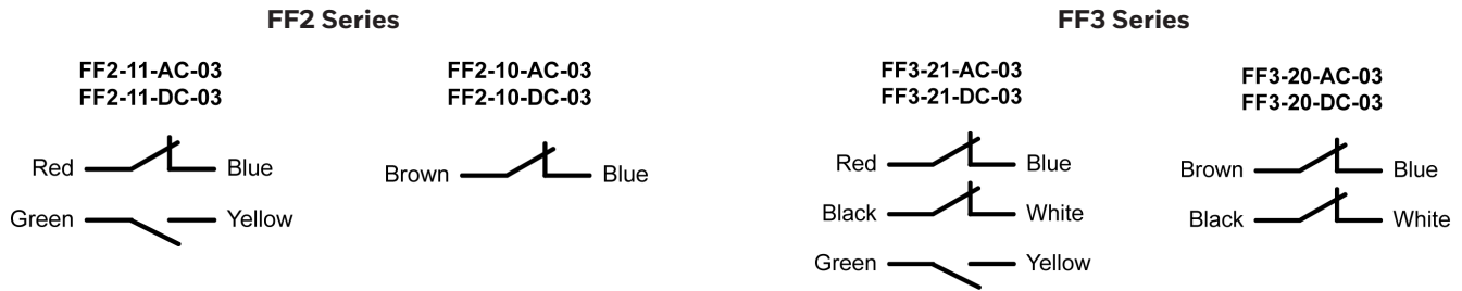
FIGURE 2. CONTACT CONFIGURATION DIAGRAMS*
