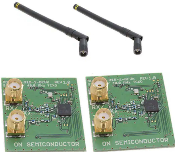
Figure 2. Content of the ADD5043-915-x-GEVK Kit
