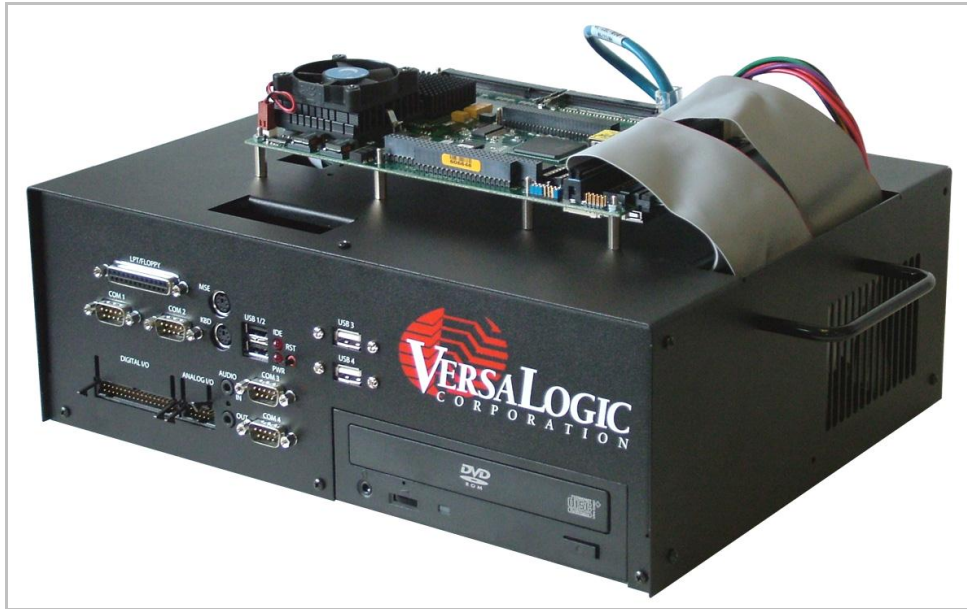
Figure 10. Example EBX Board Installation
