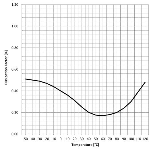
Test Equipment: E4991A or equivalent
