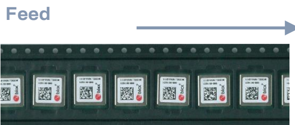
Figure 12: Orientation of NINA-B111 modules on tape
