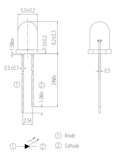
Note: Tolerances unless dimensions ±0.25mm
