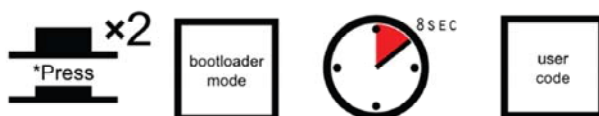
Pro Micro and Fio v3 reset functionality. Press reset twice, quickly to enter bootloader mode.
