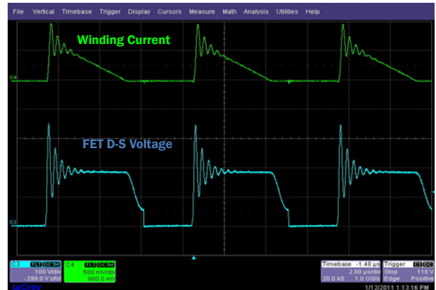
FIGURE 16. QUASI-RESONANT NEAR-ZVS SWITCHING
