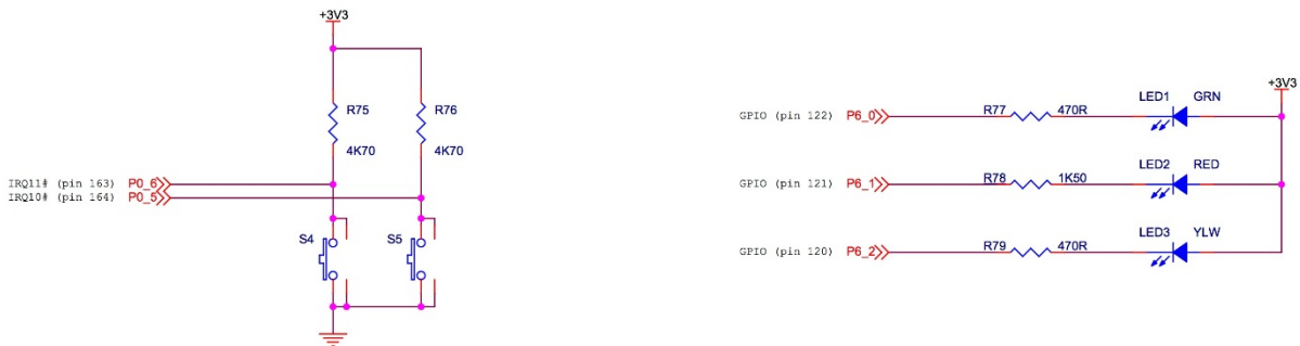
Figure 17: User buttons and LEDs
