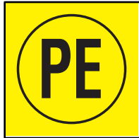
PESC*-PE Protective conductor
