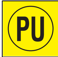
PESC*-PU Protective conductor - no earth
