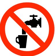
PESV*-10 Not drinking water
