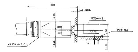
Note: Screw for Panel: M3 x 0.5 length 6 mm.
