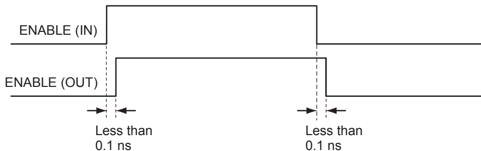
Figure 8-15 • Timing Diagram (option 1: bypasses skew circuit)
