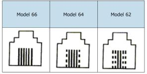
Models 64 and 62 are obtained by removing 1 pin and 2 pins, respectively, from both sides of model 66. Please check the drawing for details.
