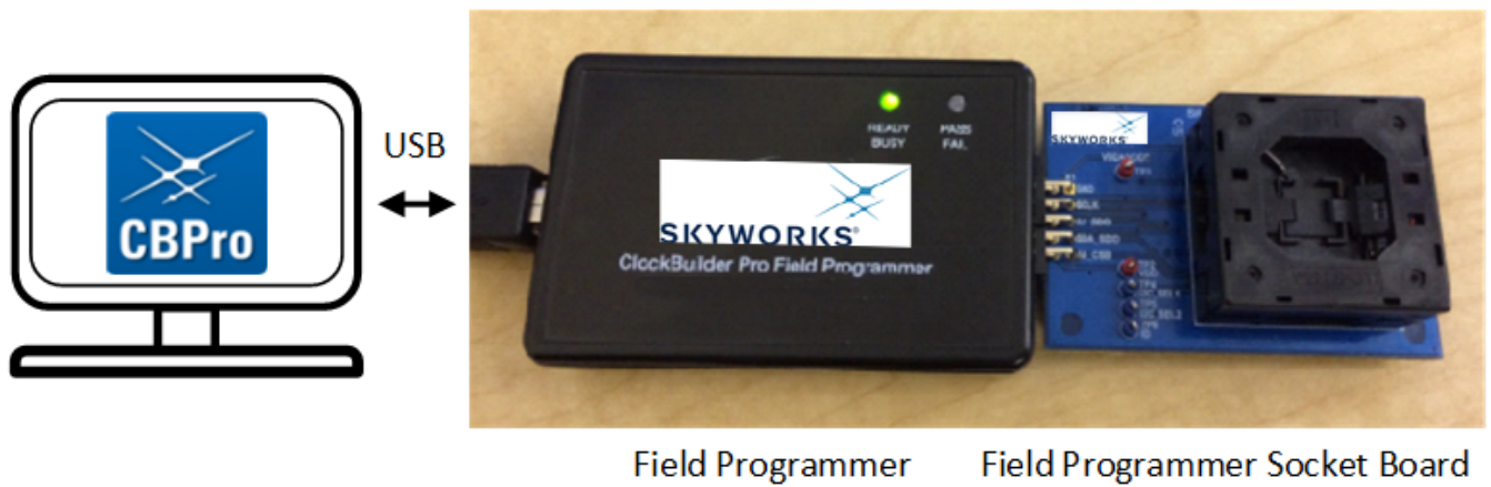
Figure 4.3. System from PC to Programming CBPROG-DONGLE Board to Field Programmer Socket Board
