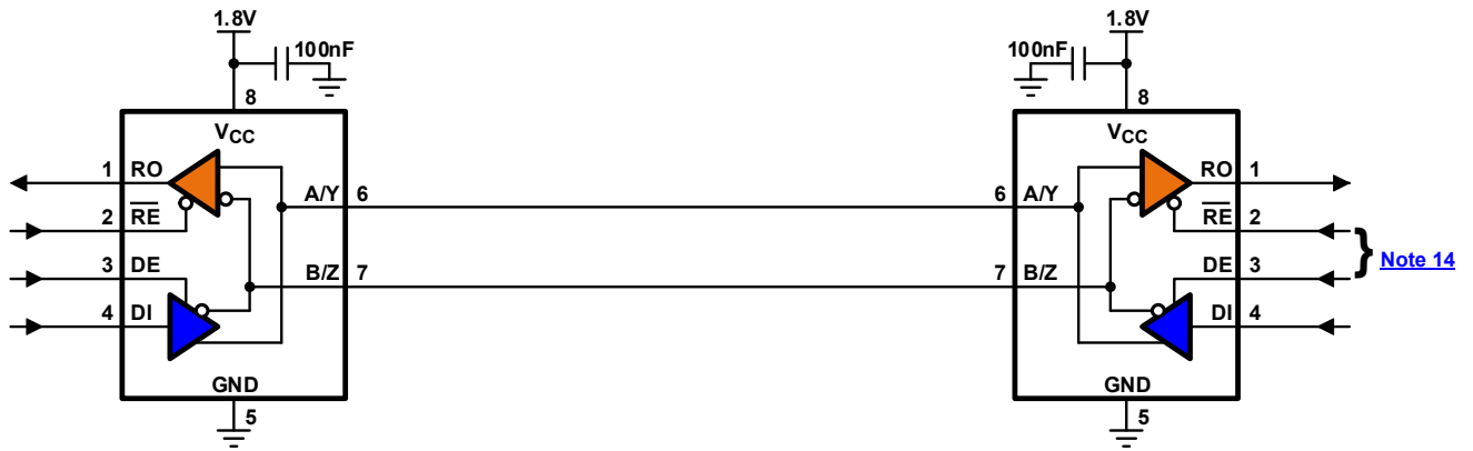
FIGURE 3. HALF DUPLEX NETWORK USING ISL32603E
