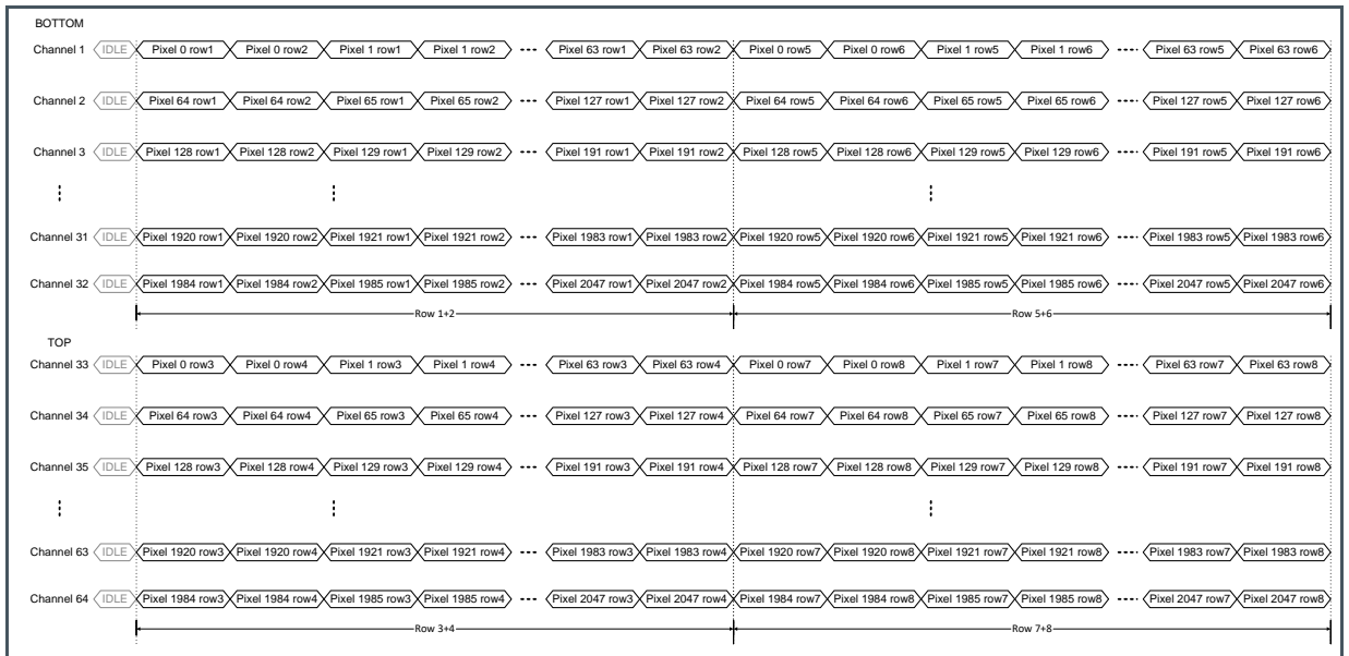
Figure 74: Pixel Remapping for Monochrome Binning
