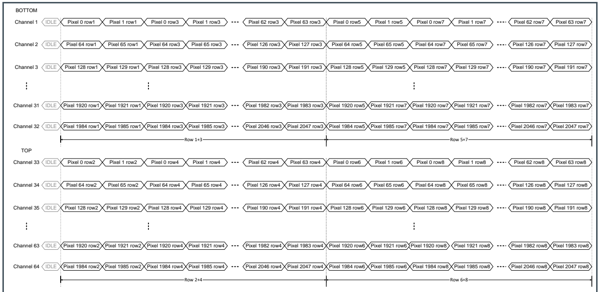
Figure 69: Pixel Remapping for Color X&Y-Subsampling
