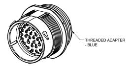
TITLE: RECEPTACLE,24-35 POS, PIN CONT., REDUCED DIA, SEAL, AHDP DWG NO: AHDPO4-24-35PR-WTA REV: A2 SH:
