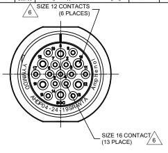
RECEP.,24-19 POS,SOCKET CONT.,REDUCED DIA. SEAL, AHDP
