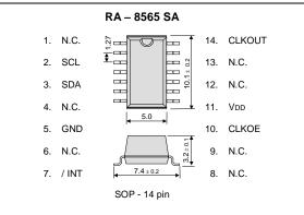
The metal case inside of the molding compound may be exposed on the top or bottom of this product. This purely cosmetic and does not have any effect on quality, reliability or electrical specs
