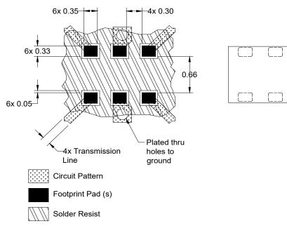
Dimensions are in Millimeters Mounting Footprint Rev C
