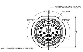
1. MATERIAL: HOUSING: THERMOPLASTIC; BLACK SEAL: SILICONE RUBBER
