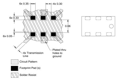
Dimensions are in Millimeters Mounting Footprint
