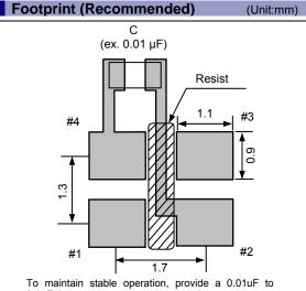
0.1uF by-pass capacitor at a location as near as possible to the power source terminal of the crystal product (between Vcc - GND).
