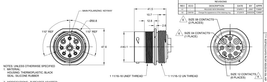
2. MODIFICATIONS: THREADED ADAPTER; REDUCED DIA, WIRE SEAL
