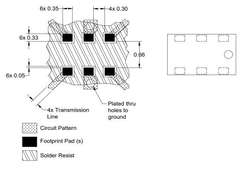
Dimensions are in Millimeters Mounting Footprint
