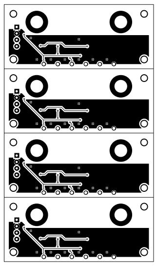
Figure 5. PCB Bottom Layer
