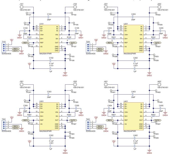
Figure 2. INA250Ax Test Board Schematic
