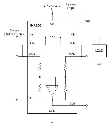
NOTE: One block diagram shown for all four EVM boards. Block diagram is functionally equivalent for all four EVM boards.
