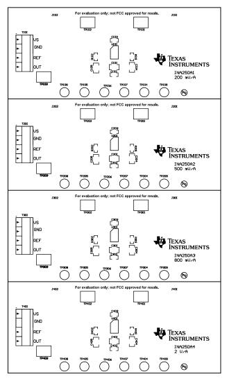
**Figure 3. PCB Component Placement**
