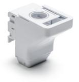
TSRP power rated surface raceway systems have an enhanced "channel and lug" mating design that provides a tighter, more secure fit between raceway lengths and fittings, enabling the system to be UL Listed for power up to 600 volts and meet UL5A and CSA 22.2.
