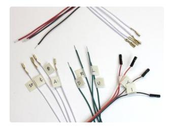
Four of the white quick-connect wires should be labeled with: A, B, ¢ and 1P. The other four quick-connect wires do not receive labels.
