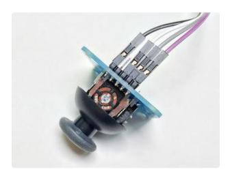
There are 5 pins on the joystick board, but only 4 jumper wires in the kit. Skip over the "Sel" pin...only the VCC, Xout, Yout and GND pins are used in Cupcade.
