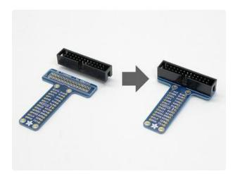
Install the male (pin) header on the Pi T-Cobbler.
