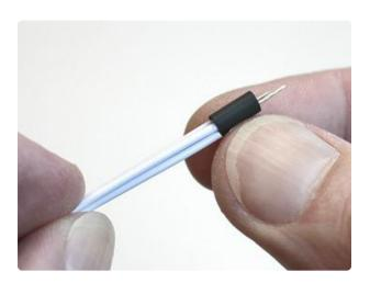
Gather up four quick-connects (the unlabeled ones) and squeeze the tips through a piece of heat-shrink tube.
