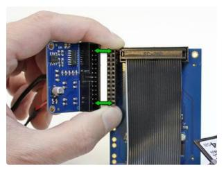
The Cupcade interface board now installs on the female header on the back of the PiTFT.
