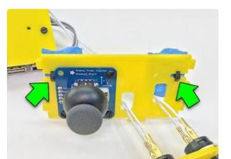
And once more for the joystick support. Two pieces of tape from behind, two nuts from the front.
