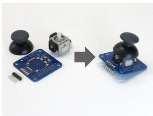
Assemble the analog thumb joystick. Some of the pins may be a little bent from shipping and need to be nudged into place. The "hat" simply presses into place.
