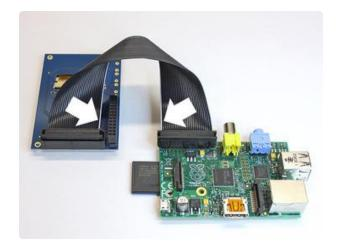
Re-install the ribbon cable between the Raspberry Pi and PiTFT, making sure the Pin 1 (white wire) is in the correct location.
