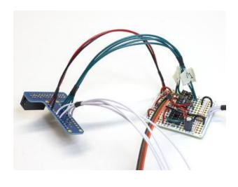
The four direction wires (U, D, L, R) can now be soldered to the appropriate positions on the Perma-Proto board. Refer to the schematic.
