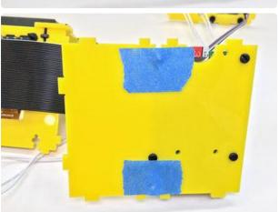
If using a Pi 3 or similar form-factor board, slide a nut into these two T-slots from the underside. The board with block them from slipping out the other side.
