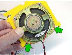
Install the speaker grille using two screws at the top.
