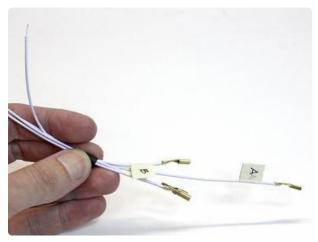
Now slide just <u>one wire</u> part way out, so we can tell it apart from the others at the bare end. Here we pulled the A wire and can identify its tail from the others.
