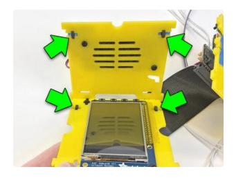
On the speaker/screen combo there's four T-slots total, two above the speaker, two above the screen.
