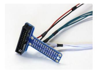
Add plain wires to the +5V and GND pins on the Cobbler (color-coded if you have them...if not, label these wires to avoid trouble).
