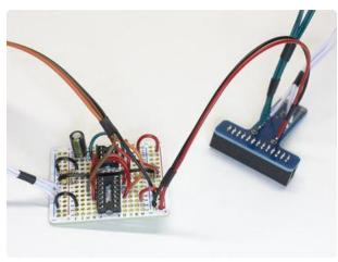
Solder the other end of the power wires to the appropriate positions on the Perma-Proto board, then heat-shrink the tubes near the ends.
