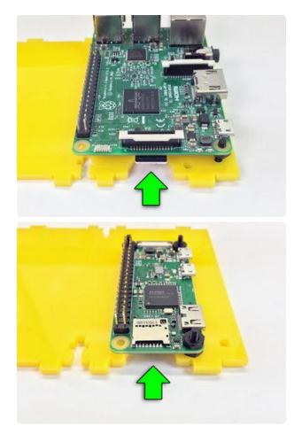
Now set the Raspberry Pi atop the screws. Only three of the board's four mounting holes are used (the fourth would interfere with other parts of the case).
