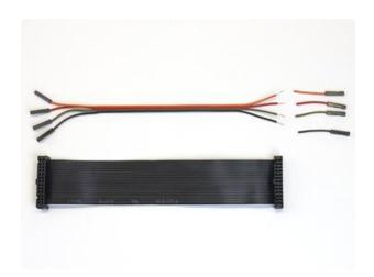
Clip one end off the 4-conductor jumper cable so it's a similar length. Separate the wires a little and strip about 1/4" of insulation.
