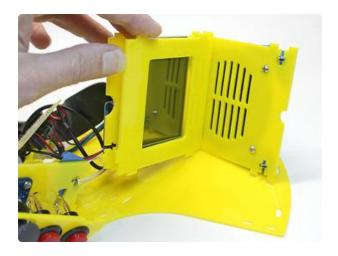
Pivot the screen support piece up slightly, fit the screen bezel into the slots on the speaker grille, and lower it all back into place.
