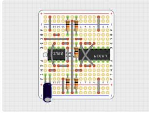
Install the 100  $\mu$ F capacitor in the position shown.
