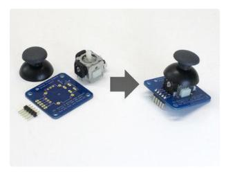
The analog thumb joystick board has a 5-pin header and quite a few pins on the stick component itself. Some of the pins may be a little bent from shipping and need to be nudged into place. The "hat" simply presses into place.
