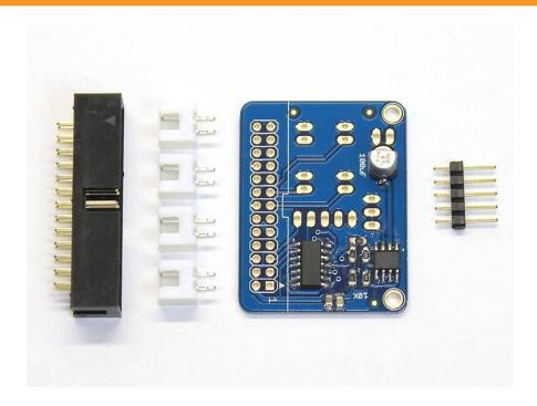
A small circuit board — specially designed just for Cupcade — features a joystick adapter circuit and a small audio amplifier. Just a few through-hole components need to be soldered.
