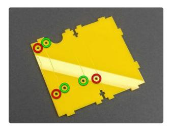
The base piece has board outlines scored on the top surface, and six mounting holes. The three "inner" holes (outlined in green) are for Raspberry Pi Zero boards, while the "outer" holes (outlined red) are for a Pi 3, Pi 2, etc. We'll use just one set or the other, depending which board you've got.
