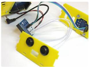
Plug the ¢ (left) and 1P (right) buttons into the corresponding sockets on the Cupcade board.
