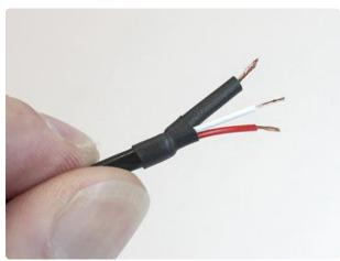
That bare copper wire on the audio cable is a problem...it might contact metal parts in the vicinity. We must insulate!
