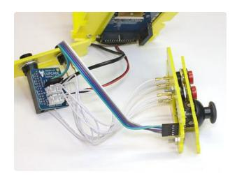
Then plug these into the corresponding sockets on the Cupcade board.
