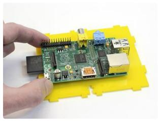
Align the mounting holes on the Raspberry Pi over these two screws.
