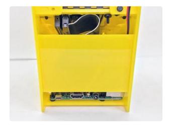
Taa-daah! The case should stand on its own now. Go around checking that all the screws are securely in place.
