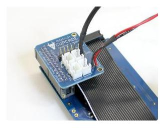
The board should be oriented to sit behind the PiTFT and ribbon cable, not hanging out over the side.
