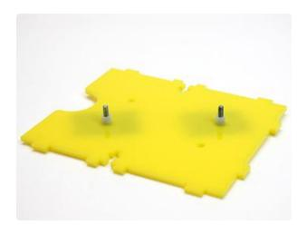
Set the piece down on your work surface with the screws pointing up, then add a nylon spacer over each screw.
