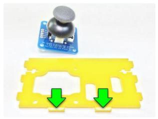
When installing the joystick on this support piece, make sure these two bumps are at the bottom.
