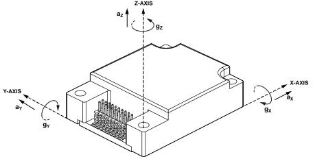
Figure 17. Inertial Sensor Direction Reference
