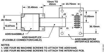
Figure 23. Physical Diagram for ADIS16445 Accessories
