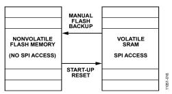
Figure 16. SRAM and Flash Memory Diagram
