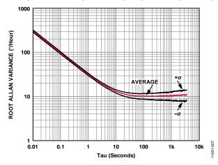
Figure 7. Gyroscope Root Allan Variance
