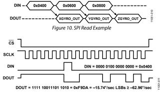
Figure 11. Example SPI Read, Second Sequence, SENS\_AVG[15:8] = 0x04
