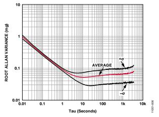
Figure 8. Accelerometer Root Allan Variance
