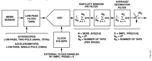
Figure 19. Sampling and Frequency Response Block Diagram
