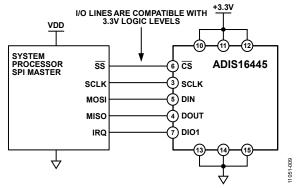
Figure 9. Electrical Connection Diagram
