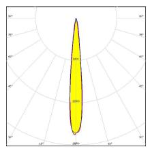
Dimensions: 16.1 mm x 16.1 mm Height: 9.70 mm ~14° spot beam. Assembly with holder and installation tape.
