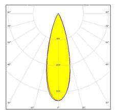
**Dimensions: 16.0 mm x 16.0 mm Height: 9.50 mm** ~30° medium beam. Assembly with holder, installation tape and location pins.
