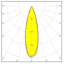
Dimensions: 16.1 mm x 16.1 mm Height: 9.70 mm ~30° medium beam optimized for CREE XP-E. Assembly with holder and
