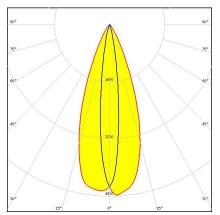
Dimensions: 16.1 mm x 16.1 mm Height: 9.70 mm ~35° + 15° oval beam. Assembly with holder and installation tape.
