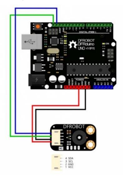
IR Thermometer Sensor-MLX90614 Wire Diagram
