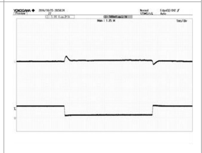
Figure 4: Dynamic response to load step 25%~75% with 0.1A/\mu S slew rate at 110/220Vac TOP: V_{out}, 500mV/div , BOTTOM: I_{out}, 5A/div, 1mS/div
