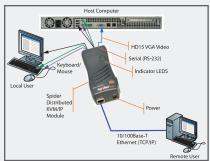
This Quick Start Guide will step you through the hardware installation and configuration in a typical environment.
