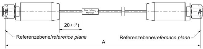
All dimensions are in mm; tolerances:  $\pm$  3mm for A  $\leq$  300 mm;  $\pm$  1% for A > 300 mm \*) If length "A"  $\leq$  90 mm marking is mount centric  $\pm$  5mm
