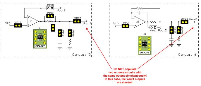
Figure 6. Wrong Connection: Outputs are Shorted
