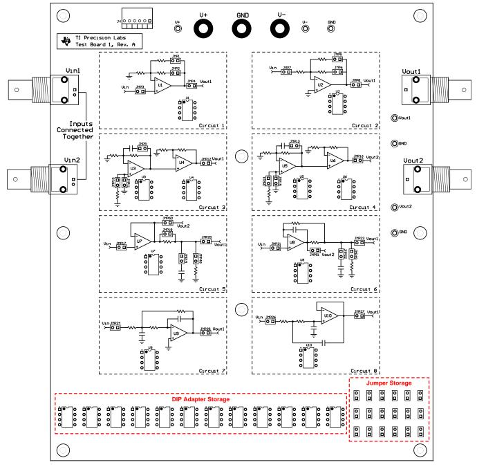
Figure 3. DIP Adaptor and Jumper Storage
