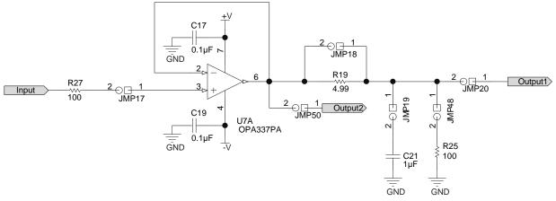
Figure 12. Circuit 5: Riso Stability Circuit
