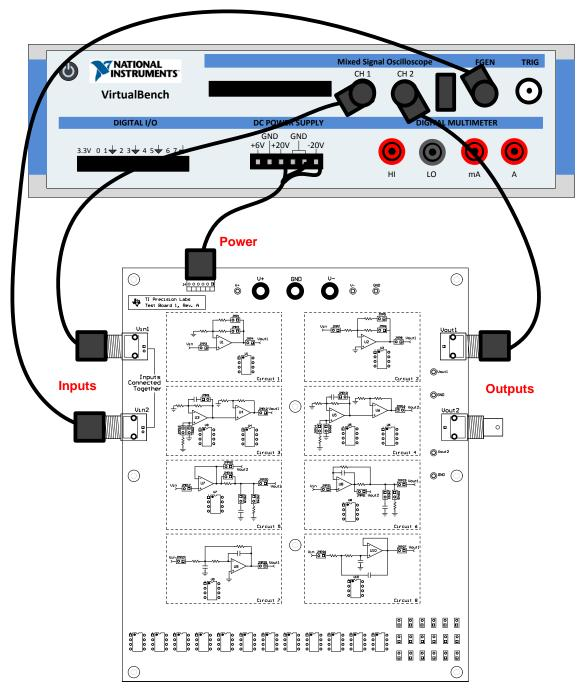
Figure 2. Input Output and Power Connections
