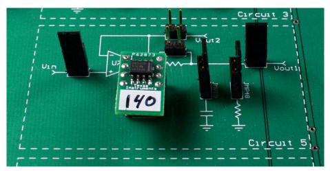
Figure 5. Configuring a Circuit
