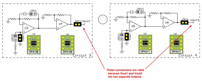
Figure 7. Correct Connection: Outputs are Connected to Separate BNC Connectors
