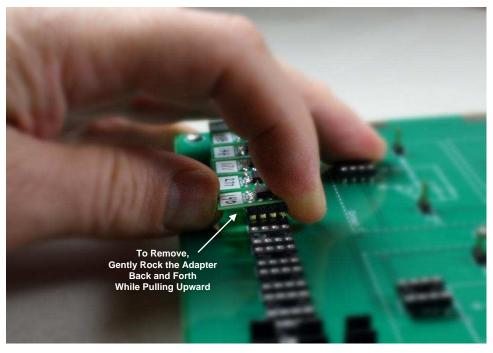
Figure 4. Removing the DIP Adaptor
