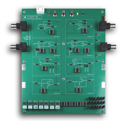
Figure 1. Hardware included with TI-PLABS-AMP-EVM Kit
