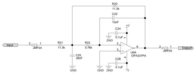
Figure 14. Circuit 7: Multiple-Feedback LPF
