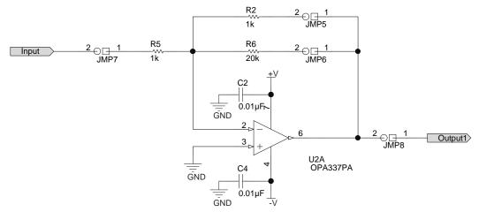
Figure 9. Circuit 2: Inverting Amplifier
