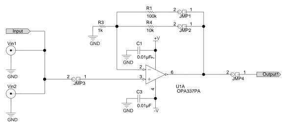
Figure 8. Circuit 1: Noninverting Amplifier
