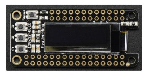
The OLED FeatherWing plugs into any Feather and adds a cute little display. To make it as cross-platform compatible as possible, we use only I2C to control the display. This is not as fast as SPI but it uses only two pins, can share the I2C bus and is fine for the small 128x32 pixel OLED.
