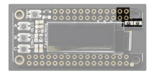
The cute little OLED does all of the data transfer over the I2C pins, highlighed above SDA and SCL. No other pins are required. There are two 2.2K pullups to 3V on each.
