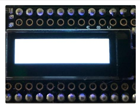
Next we will create a smaller black rectangle. The easiest way to do this is the create a new bitmap that is a little smaller than the full screen with a single color of  $0 \times 0000$  00, which is black, and place it in a specific location. In this case, we will create a bitmap that is 5 pixels smaller on each side. The screen we're using here is  $128 \times 32$  and we have the border set to 5, so we'll want to subtract 10 from each of those numbers.
