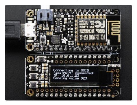
These displays are small, only about 1" diagonal, but very readable due to the high contrast of an OLED display. This screen is made of 128x32 individual white OLED
