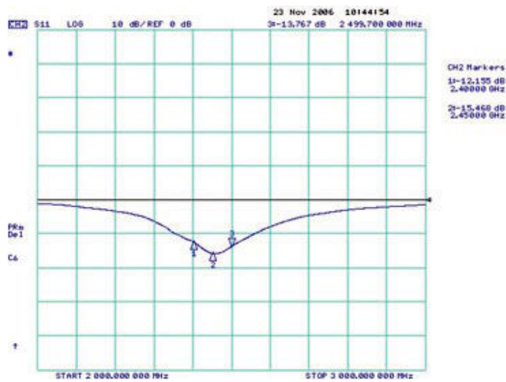
Antenna VSWR on Test Board
