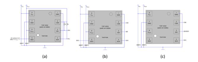
Picture 12: Connection diagrams for (a) I<sup>2</sup>C, (b) 4-wire SPI, and (c) 3-wire SPI
