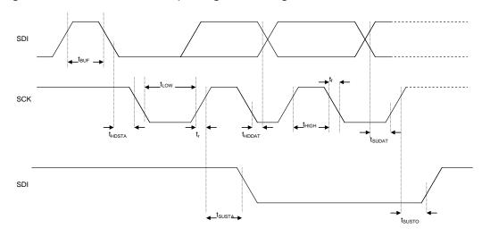
Picture 9: I<sup>2</sup>C timing diagram
