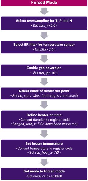
Picture 2: Sensor configuration flow
