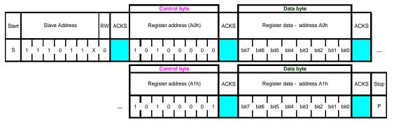
Picture 4: I<sup>2</sup>C multiple byte write (not auto-incremented)
