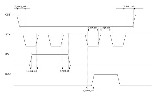
Picture 10: SPI timing diagram
