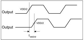
FIGURE 1-2: Output-to-Output Skew.
